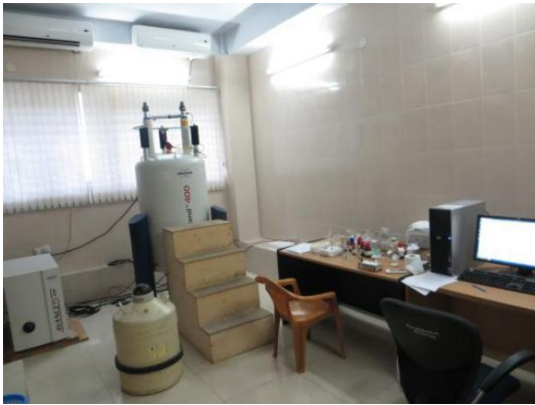
Nuclear Magnetic Resonance Spectrometer
